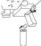
Position the cartridge inside the cartridge holder and slowly rotate the cartridge to the right until it stops.
