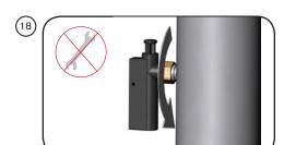
Align connections by rotating ring clamp (if equipped) to push lamp plug onto end of lamp. clamp
