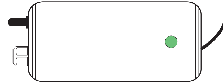
Green LED indicates UV lamp "ON".
