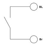
The reed contact is electrically insulated (class II) and integrated into a plastic housing. When affixing the supply cable to the flow switch, be sure to not expose the cable to excessive tension (max. 15 N).
