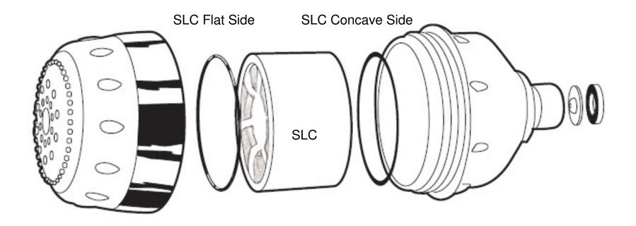
To help get a better grip on the housing, rubber gloves are recommended. Remember to lubricate inside O-rings with each filter cartridge change.
