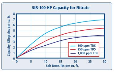
Capacity and leakage based on  $10\% \text{ NO}_3$  and  $40\% \text{ SO}_4$  in the feed and  $44 \text{ ppm NO}_3$  endpoint (all as CaCO<sub>3</sub>). Capacity and leakage are for nitrate alone. TDS is for total anions as CaCO<sub>3</sub>. No engineering downgrade has been applied.
