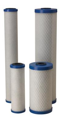
Pentek® EP Series Carbon Block Cartridges are manufactured using a process that yields a cartridge with a nominal 5-micron filtration rating and high dirt-holding capacity. A high porosity design helps prevent the cartridge from plugging before its adsorption capacity is exhausted, maximizing the utilization of the carbon while maintaining low pressure drop.
