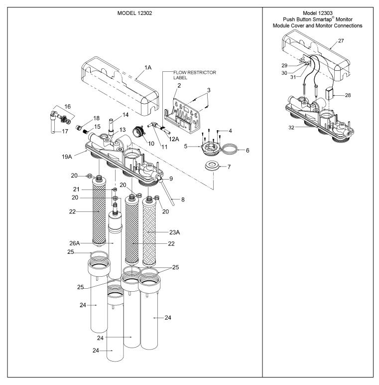
Figure 10.B: Exploded Schematic, 12302 and 12303 Model Series
