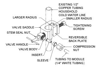
Figure 3: Saddle-Tapping Valve Assembly P/N 34900013 installed on 1/2" Copper Tubing
