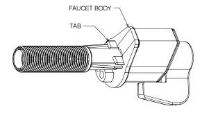
Figure 8: Faucet Locator Tabs and Air Gap.
