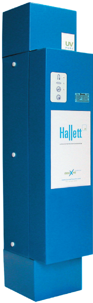
Hallett 30 1" 30 USGPM (114 L/min) (6.81 m³/h) 40 mJ/cm² @ 75% UVT
