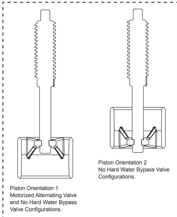
V3076 MAV and WS2 valves shown. Diagram is typical for WS1.5, WS2L, or WS2 valves using V3071 or V3076 piston style MAV's and regenerating with hard water.
