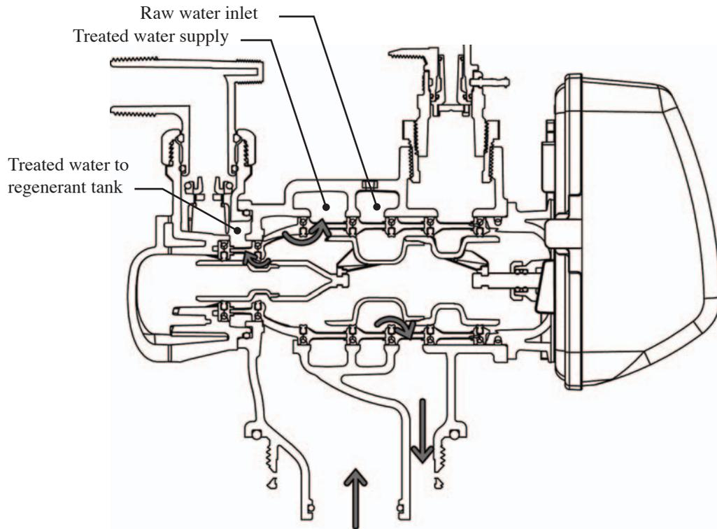
**WS1.5 Drive Cap Assembly, Downflow Piston, Upflow Piston, Regenerant Piston, Spacer Stack Assembly and Main Body**
