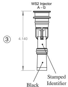
\*\* V3010-2X-15X Injectors contain a V3010-2-15 WS2 injector adapter with a WS1.5 injector inside
