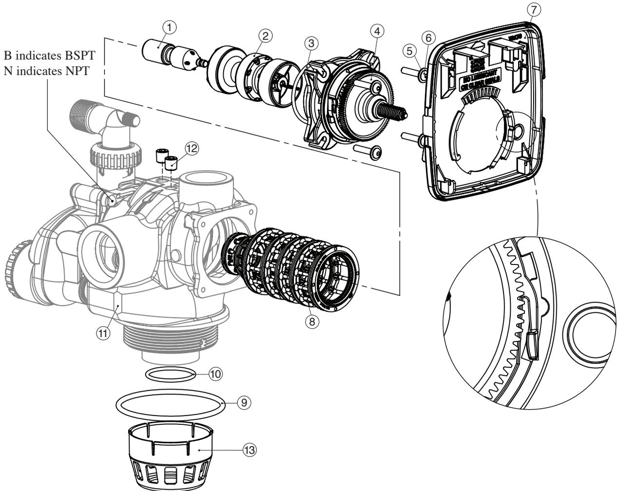
**WS2 Quick Connect Drive Cap Assembly, Downflow or Upflow Piston, Regenerant Piston, Downflow or Upflow Spacer Stack Assembly and Main Body**
