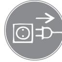
Disconnect from electrical power prior to servicing the valve.
