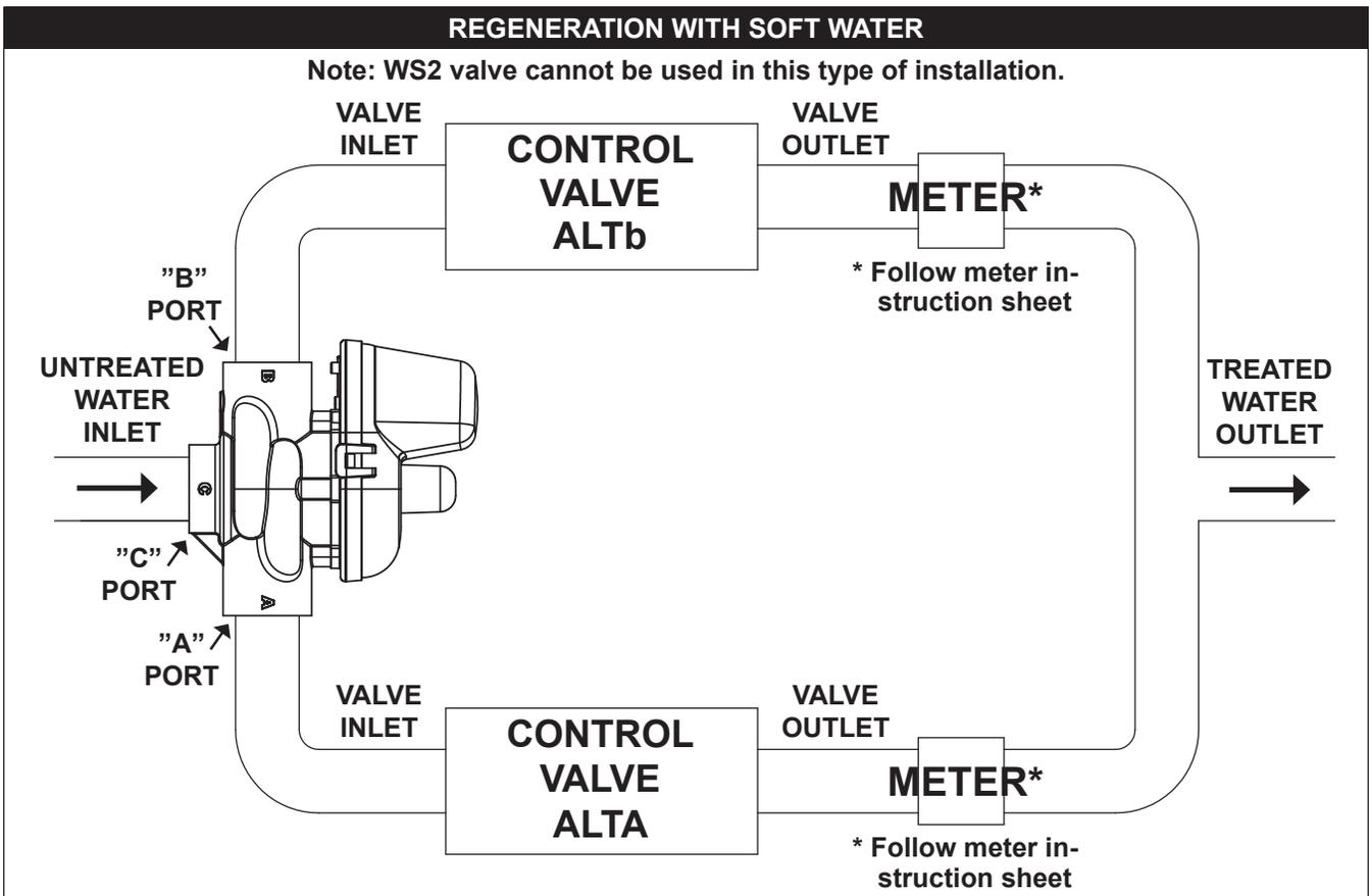
1.5" Piston Style MAV's (See Installation Instructions on Motorized Alternating Valves)
