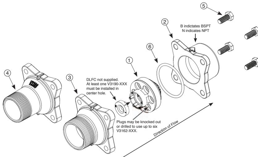
**Drain Line Flow Control Washers**
