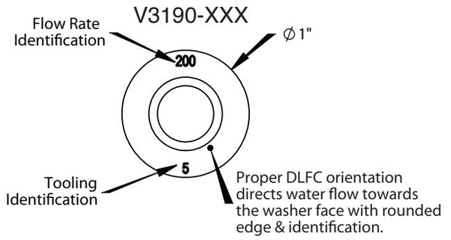
All DLFC housings ship without DLFC installed.
