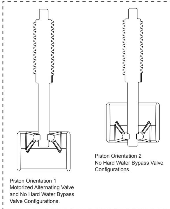
**2" Piston Style MAV's (See Installation Instructions on Motorized Alternating Valves)**
