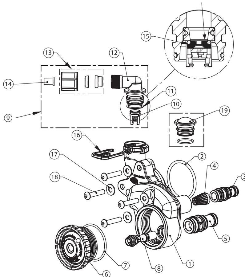
**WS2 Injector Valve Body, Refill Flow Control and Injector**
