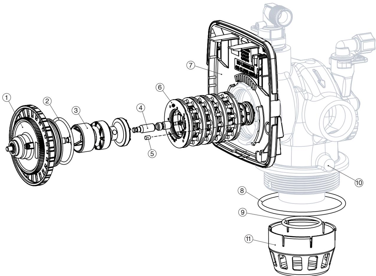
**WS2 Drive Cap Assembly, Downflow or Upflow Piston, Regenerant Piston,
