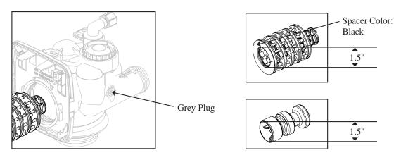
WS1.25CS with 32mm Distributor Tube Opening Identification
