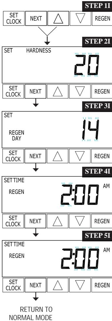
**STEP 1I** - Press NEXT and ▲ simultaneously for 3 seconds.
