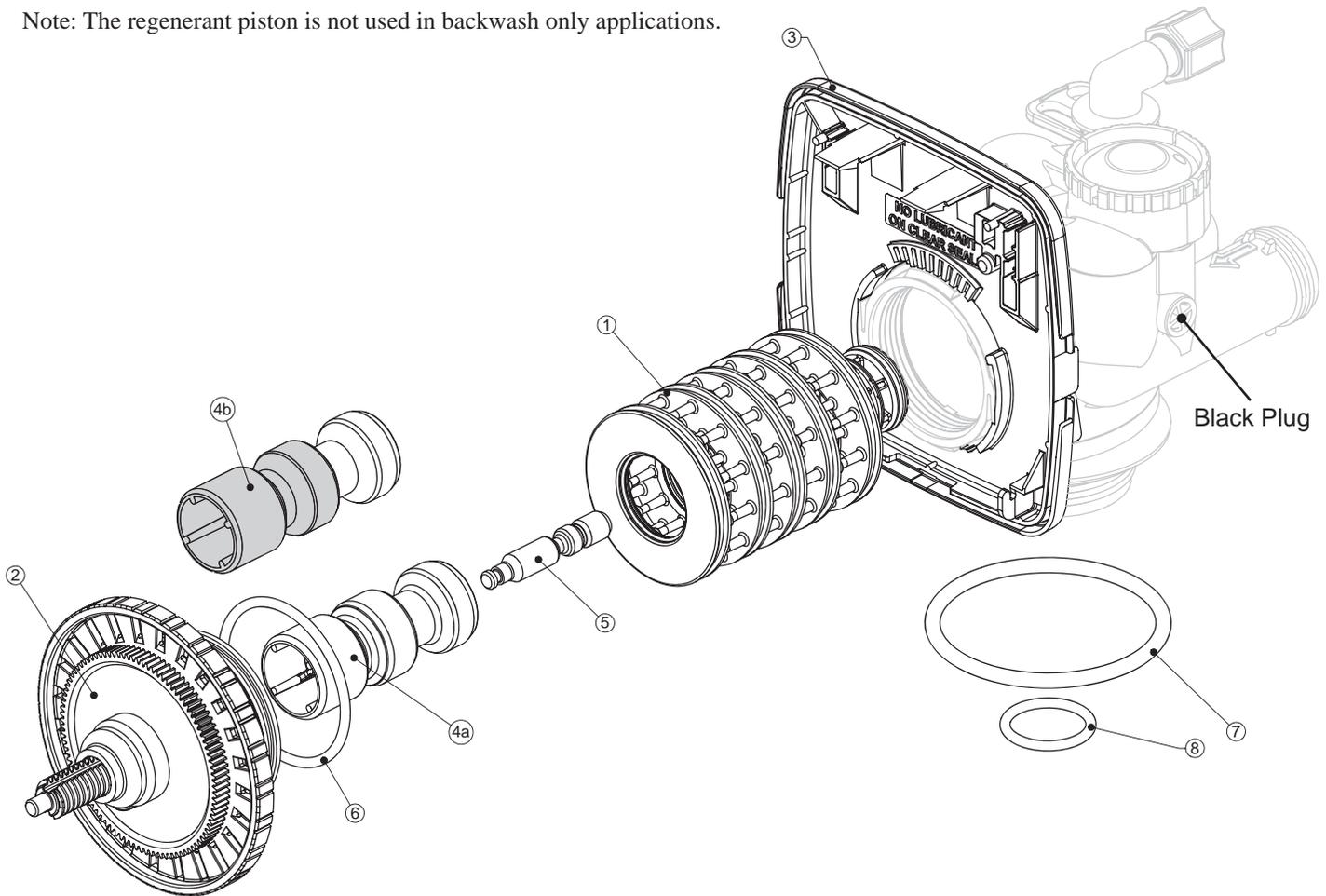
**WS1.25CS Drive Cap Assembly, Downflow Piston, Regenerant Piston and Spacer Stack Assembly**
