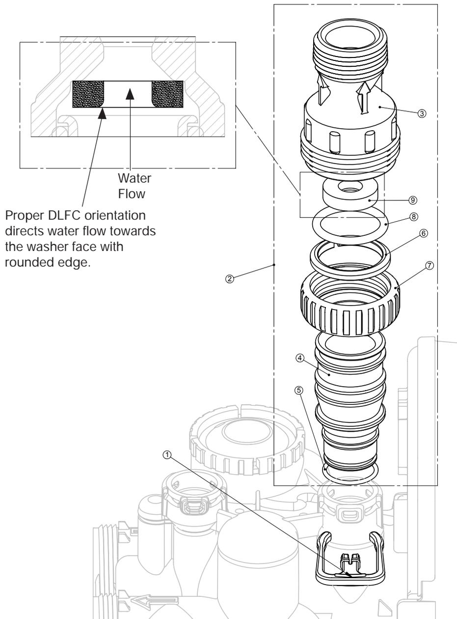
**Water Meter, Meter Plug and Mixing Valve**
