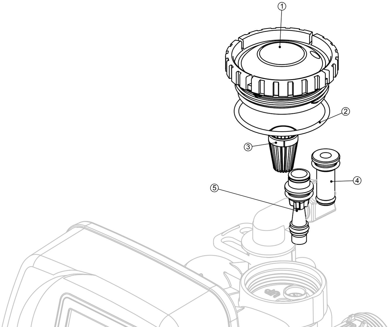
**Refill Flow Control Assembly and Refill Port Plug**
