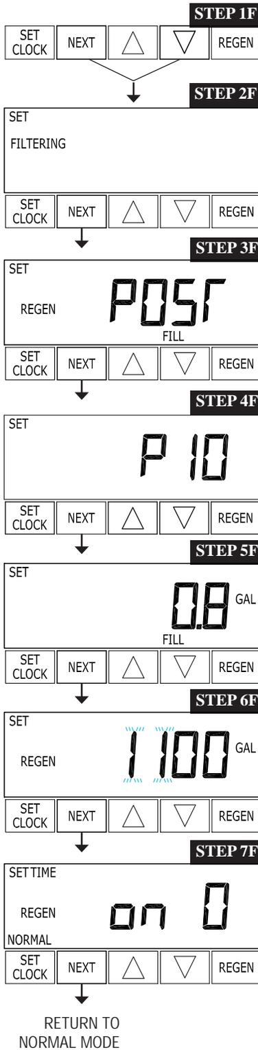
**STEP 1F** – Press NEXT and simultaneously for 3 seconds. If screen in step 2F does not appear in 5 seconds the lock on the valve is activated. To unlock press , NEXT, , and SET CLOCK in sequence, then press NEXT and simultaneously for 3 seconds.
