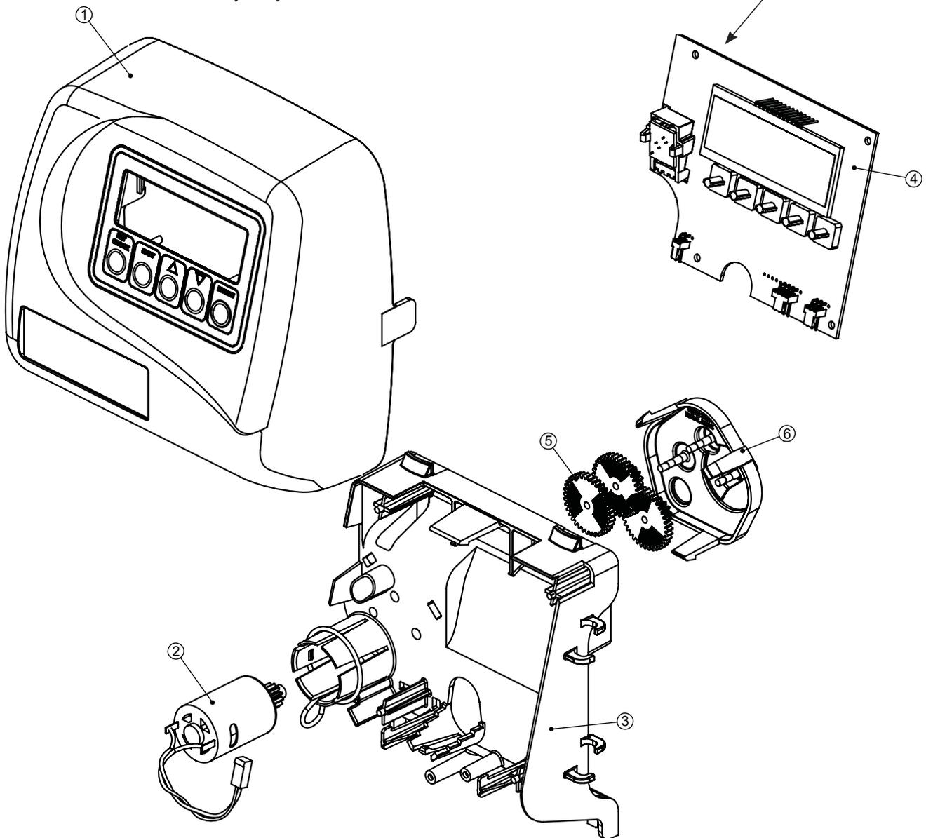
**WS1CS Drive Cap Assembly, Downflow Piston, Upflow Piston, Regenerant Piston and Spacer Stack Assembly**
