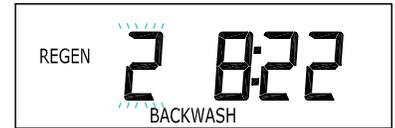
When the system begins to regenerate, the display will change to include information about the step of the regeneration process and the time remaining for that step to be completed. The system runs through the steps automatically and will reset itself to provide treated water when the regeneration has been completed.
