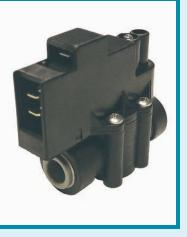
Our Pressure and Vacuum Switches (PSW and VSW Series) provide a full range of in-line pressure sensing electrical switches. These switches, typically mounted near a hydropneumatic holding tank, automatically control the system pump and/or solenoid valve as required. They can also be used to enable hydraulic shut-off valves to operate reliably and positively.
