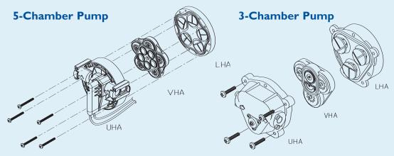
UHA: Upper Housing Assembly • VHA: Valve Housing Assembly • LHA: Lower Housing Assembly
